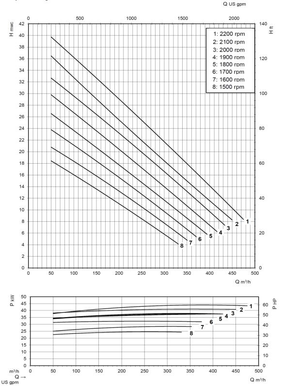
Pump performance curves are bases on the speed of the powerpack diesel engine.
